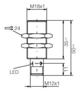
**Inductive Sensors** BES M18MF1-PSC50A-S04G-W M18x1 x 52 normally-open Sn=5mm shielded Factor 1
